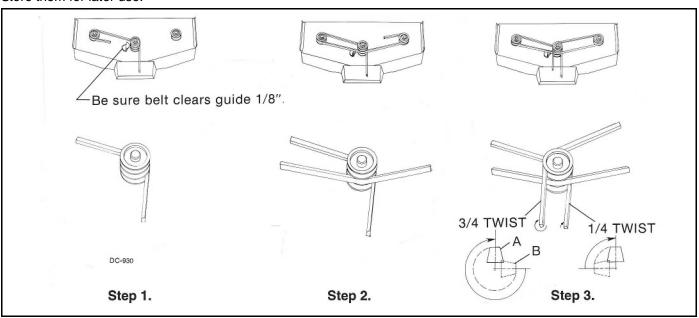
Figure 18. Belt Installation
